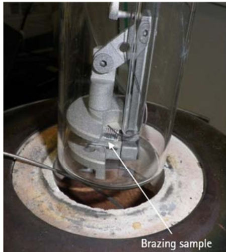
Figure 12. Brazing jig with brazing sample in the reaction vessel.
