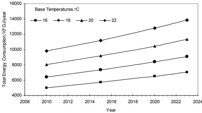
Fig. 4. The predicted total energy consumption for insulated buildings or different base temperatures in a heating season.
