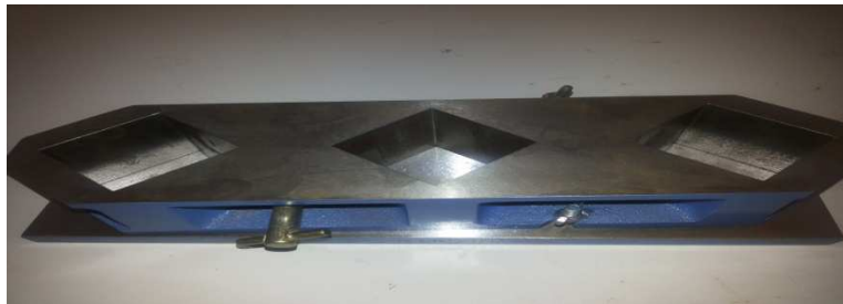
Figure 3.1. 3-gang Mould.
