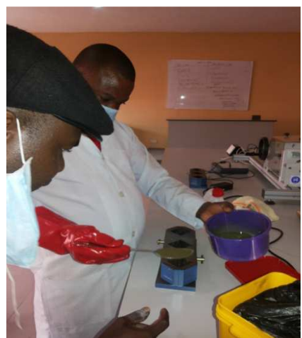
Figure 3.5. Composites Lamination in Progress.
