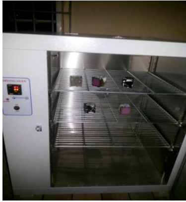
Figure 3.10. Conventional Oven Curing in Progress.
