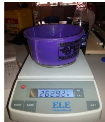
Figure 3.2. Conducting fillers measurement in progress.
