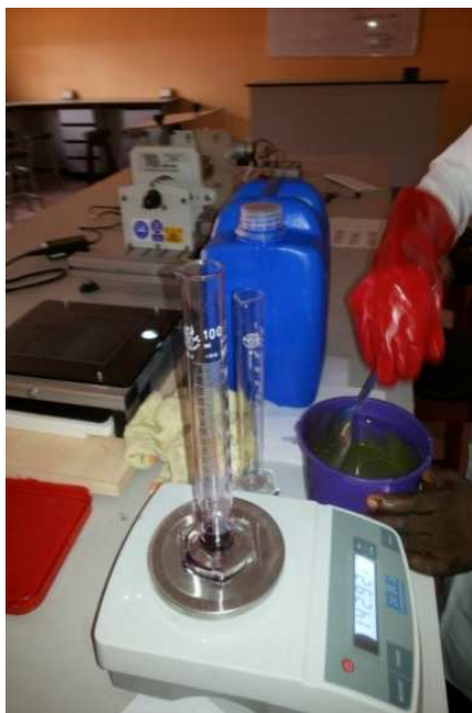
Figure 3.3. Hardeners measurement in progress.
