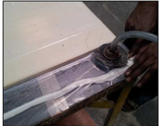
Figure 1. Sandwich panel fabricated using vacuum bagging technique.
