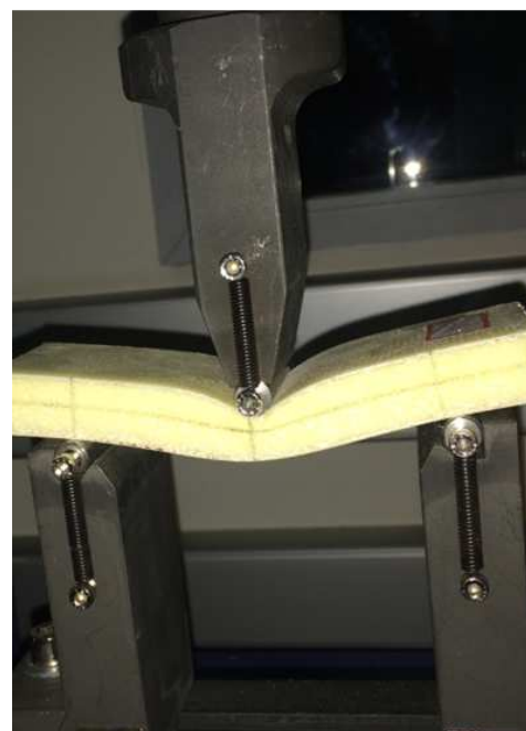
Figure 6. Flexural testing of sandwich beam.
