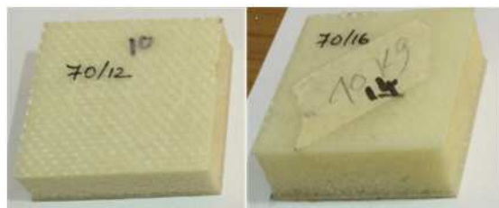
Figure 2. Flatwise compressive test specimen.
