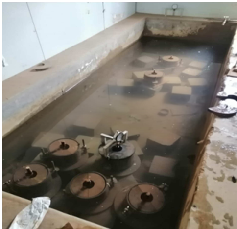
Figure 2. Soaked CBR samples.
